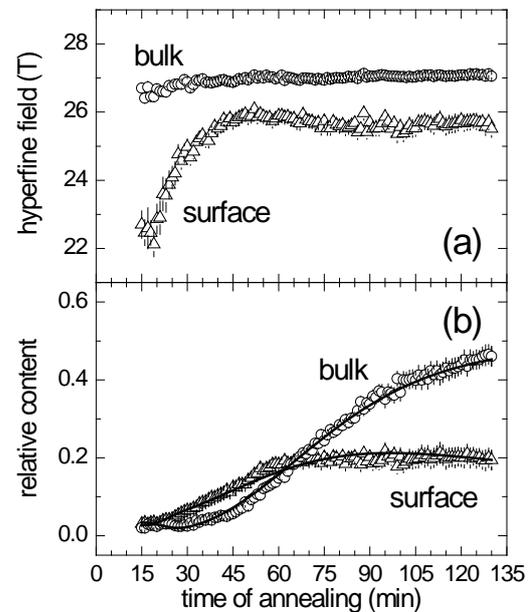
**Fig. 5** Magnetic hyperfine fields (a) and the relative contents (b) of the bulk and surface iron atoms plotted against the time of annealing at  $470^\circ\text{C}$
