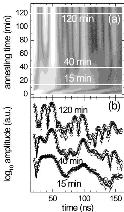
**Fig. 4** Contour plot (a) obtained from isothermal NFS experiment upon  $\text{Fe}_{90}\text{Zr}_7\text{B}_3$  MG and several selected records (b) obtained after the indicated times of annealing. Solid lines are fits to the experimental data (open symbols)
