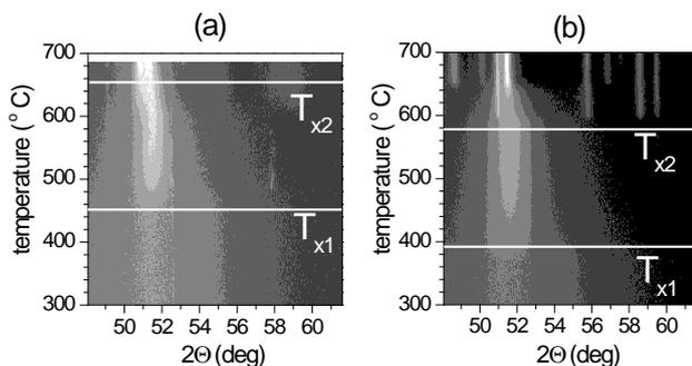
**Fig. 1** Contour plots of diffractograms from  $(\text{Fe}_{1-x}\text{Co}_x)_{76}\text{Mo}_8\text{Cu}_1\text{B}_{15}$  alloy for  $x = 0$  (a) and  $x = 0.25$  (b). Crystallization temperatures  $T_{x1}$  and  $T_{x2}$  are indicated by horizontal lines
