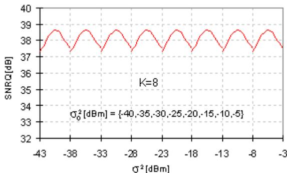
**Fig. 3** SNRQ for bit rate  $R = 7,5$ ,  $N_i = 4096$ ,  $R_0 = 7.525$ ,  $M=60$  and for eight quantizers designed for different values of  $\sigma_0$
