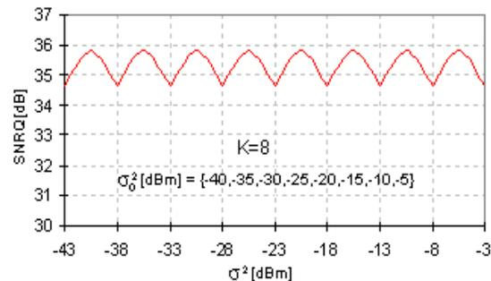
**Fig. 5** SNRQ for bit rate  $R = 7$ ,  $R_0 = 7.025$ ,  $M=60$ ,  $N_i = \text{const}$  and for eight quantizers designed for different values of  $\sigma_0$
