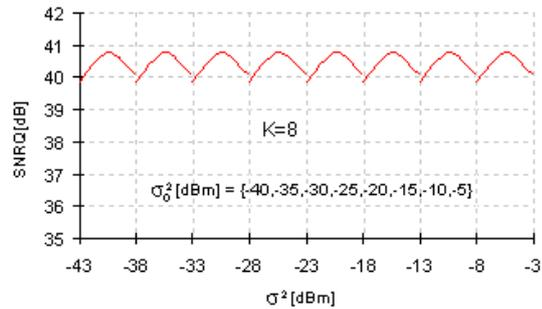
**Fig. 4** SNRQ for bit rate  $R = 7,5$ ,  $R_0 = 7.525$ ,  $M=60$  optimum number of output points  $N_i$  and for eight quantizers designed for different values of  $\sigma_0$
