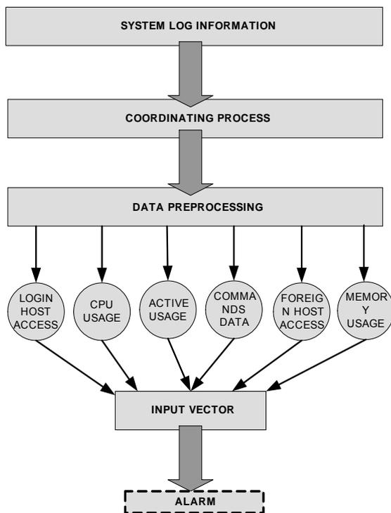
**Fig. 5** Structure of an Automated User Behavior Anomaly Detection System
