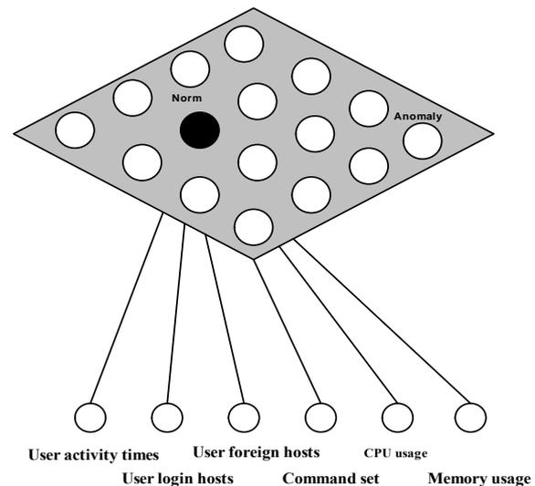
**Fig. 6** Form of the designed SOM architecture
