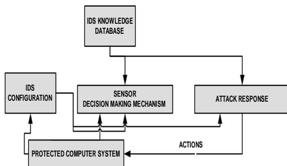
Fig. 3 Intrusion detection system
