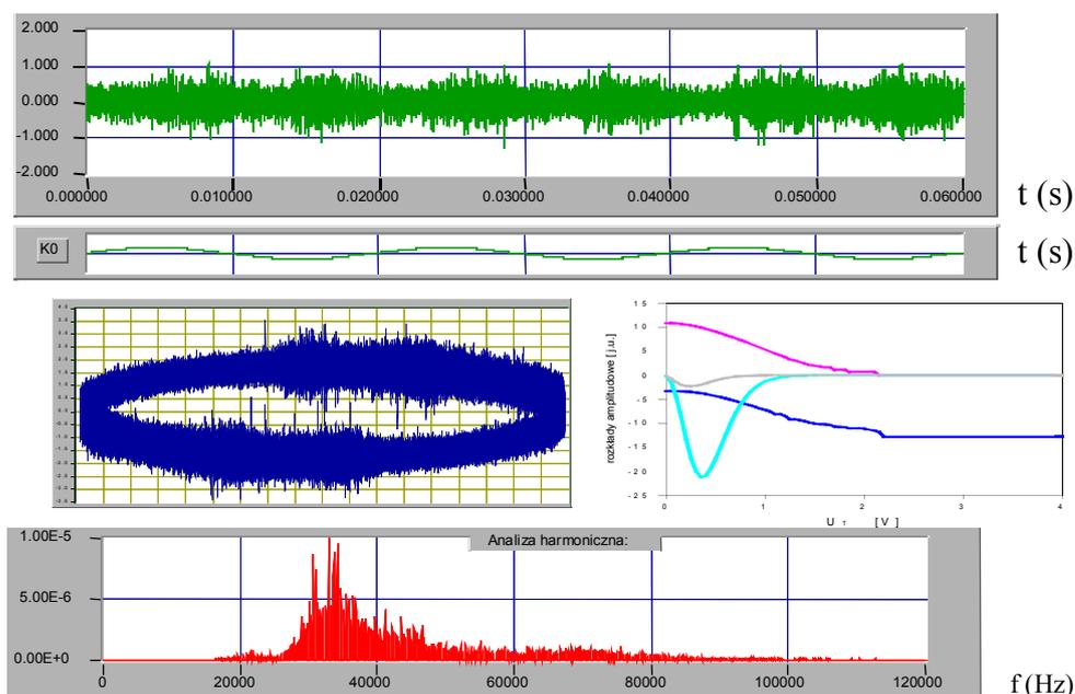
Fig. 2 An acoustic image of registered PD (exemplary measuring situation)
