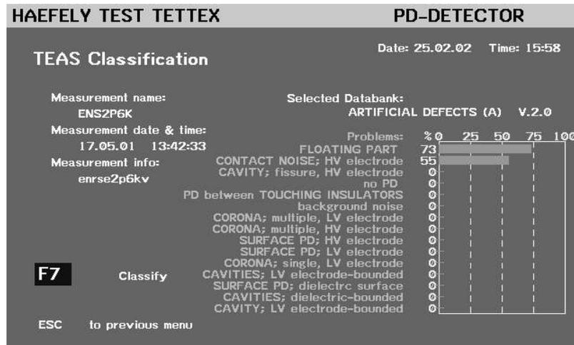
**Fig. 6** An exemplary result of statistical analysis regarding PDs registered during the test of one generator bar in the firm ELEKTROSERWIS (Lubliniec)
