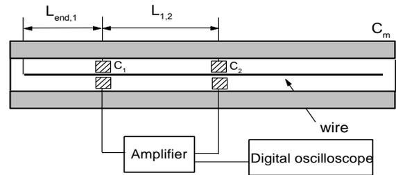
**Fig. 1** Schematic diagram of the arrangement of Sixtus-Tonks experiment.  $C_m$  is 41 cm long magnetizing coil,  $C_1$ ,  $C_2$  are 5 mm long pick-up coils. Induced signal in pick-up coils is 10 000 times magnified.
