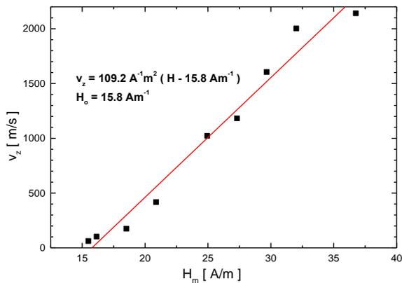
**Fig. 5** The measured dependence of the axial velocity  $v_z$  of the propagating reverse domain wall on the intensity of the external driving field  $H_m$  fitted by the theoretical straight line  $v_z = S (H_m - H_0)$ .
