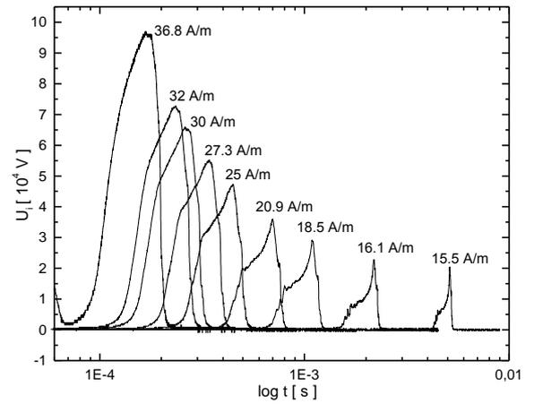
**Fig. 4** Induced impulses during the propagation of the reverse domain wall at displayed external driving field  $H_m$ . The first type of impulses recorded at lower fields ( $H_m = 15.5 \text{ A/m}, \dots, 25 \text{ A/m}$ ) corresponds to the propagation of the conical reverse domain wall. The second type of impulses recorded at higher fields ( $H_m > 25 \text{ A/m}$ ) displays a shape transformation of the propagating reverse domain wall to a quasi-planar wall (see Fig. 2, 3).
