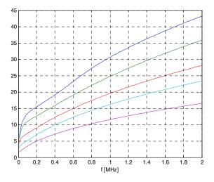
**Fig. 1** Typical relations between frequency and relative attenuation for lines with quad arrangement (local telecommunication cables) – core diameters from upside: 0.32, 0.4, 0.5, 0.63 and 0.9 mm
