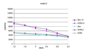
Fig. 3 Comparison of simulation results with measured speeds
