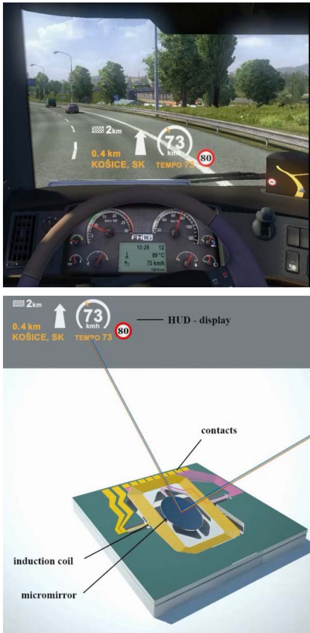
Fig. 5 HUD (head-up display) utilizing MEMS scanner that visualize the navigation, velocity and road signs information on the front window
