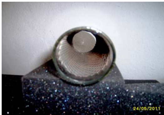
Fig. 3 Cylindrical DBD reactor with internal mesh electrode
