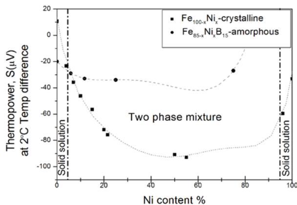
Fig 2 The evaluation of thermopower in the case of crystalline and amorphous state alloys at 2C temp difference
