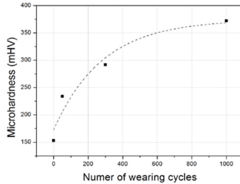
**Fig. 6** The evaluation of microhardness versus the wearing cycles in C45 steel
