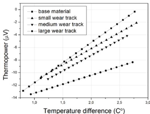
**Fig. 5** Thermopower characteristics of C45 samples with increasing wear degrees
