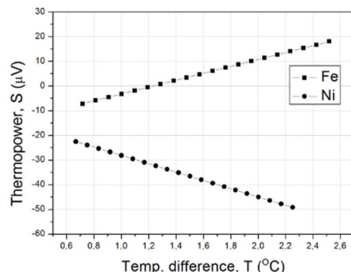
Fig. 1 TEP of Fe and Ni metals
