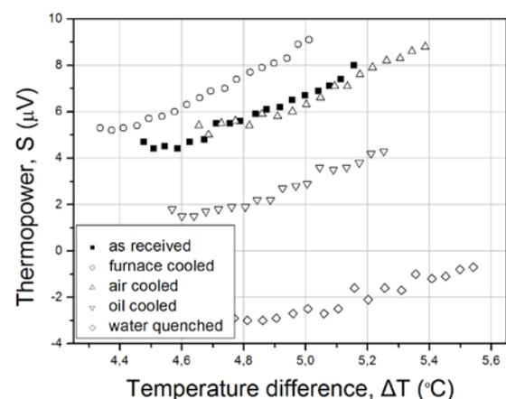
Fig3 Influence of heat treatment on the evaluation of thermopower in C45 steel [5]
