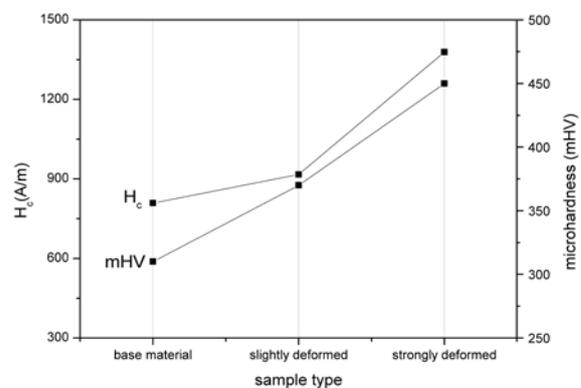
**Fig. 7** Static coercivity ( $H_c$ ) and microhardness (mHV) versus deformation state in a rail-material
