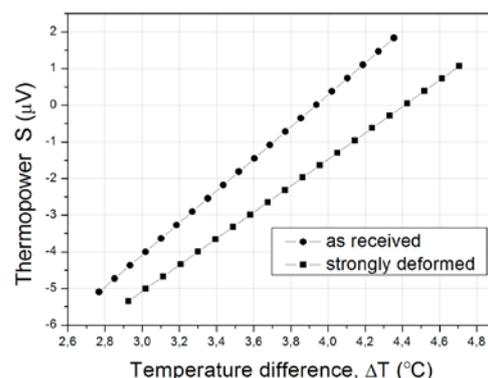
**Fig. 8** Thermopower measured on rail-material samples with different deformation states
