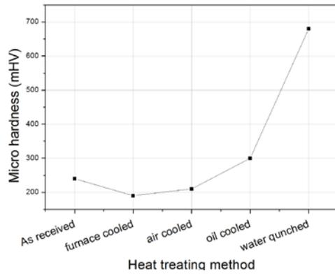
**Fig. 4** The evaluation of micro hardness versus the cooling rate in C45 steel
