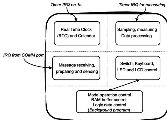
**Fig. 2** Block diagram MMS SW structure (State Chart)
