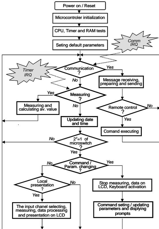
Fig. 3 MMS Working Program block diagram
