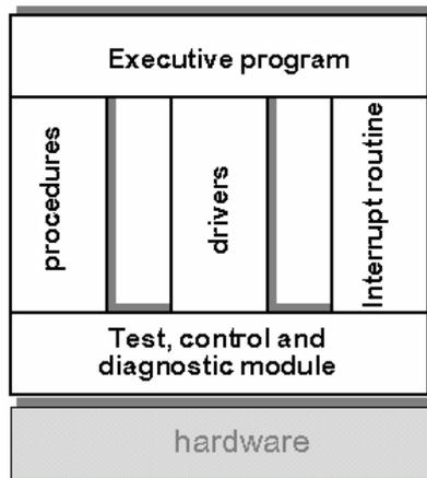
Fig. 1 MMS Software block diagram
