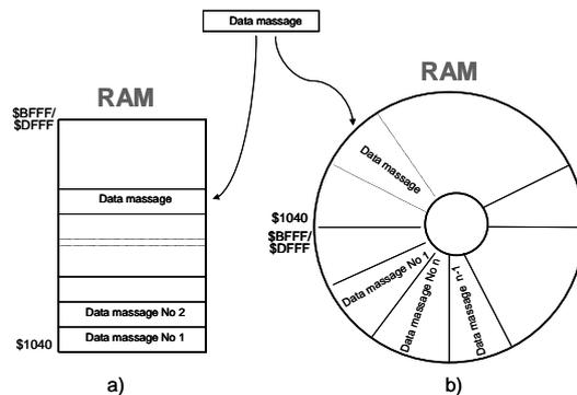
Fig. 5 Storing data in RAM: a) Mailbox Mechanism, b) Ring Buffer Principles
