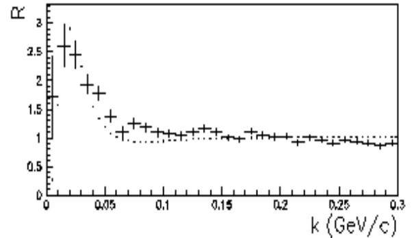
**Fig. 3** Proton - proton correlation function for dp reaction. The curve represents the theoretical calculation.
